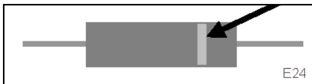
Fig. 2 Marking of the cathode
