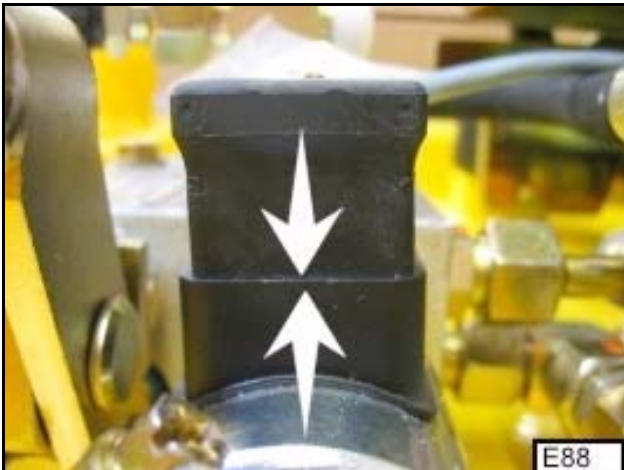
Fig. 14 Correctly installed plug without gap
