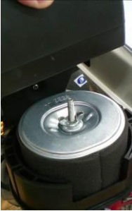
1 REMOVE THE AIR FILTER COVER
