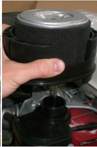
2 REMOVE THE AIR FILTER
