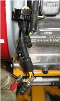
1 DISCONNECT THE BLACK WIRE FROM THE SPARK
